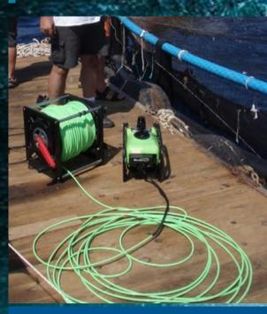
Mini OCROVs—vehicles with submersible weight between 4.5 kg and 32 kg
