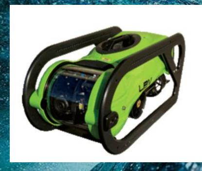
**Class I** - Observation ROVs Small vehicles fitted with camera, lights and a sonar only.
