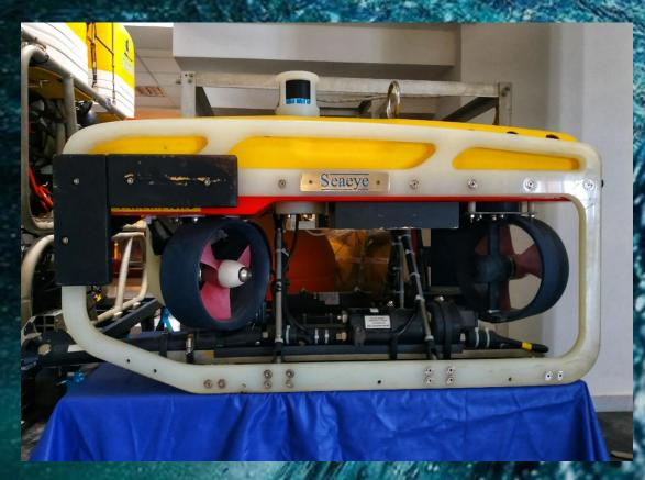
Depth rating 300 m 1000 mm Length 500 mm Height Width 600 mm Weight in air 60 kg Payload 14 kg Forward thrust 40 kgf Lateral thrust 23 kgf Vertical thrust 13 kgf 3 kn Speed > Thruster type \$1-MCT01 Horizontal thrusters Vertical thrusters Auto-depth Auto-heading Video channels Video transmission STP/FO
