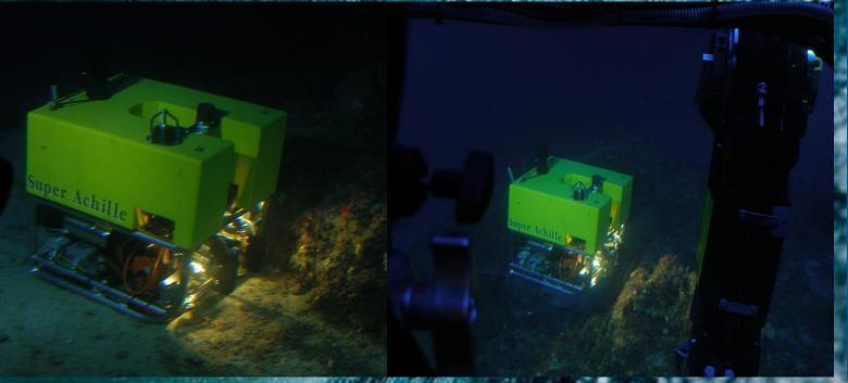
Depth rating 1000 m Length: 720mm 600mm Width: 510 mm Height:
