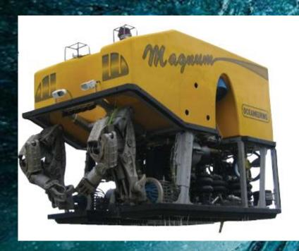
**Standard work class:** These vehicles are in the 100 -200 hp range typically used in drill support or light construction
